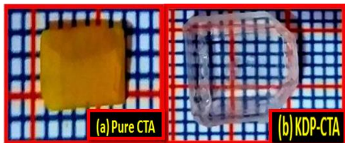
Figure 1. (a) Pure CTA (b) KDP doped CTA crystal
